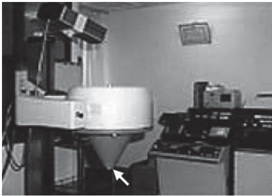
Fig. 1. Pinhole scanner showing pinhole collimator inserted at the top of the cone shield assembly. The optimum aperture size is 4 mm
